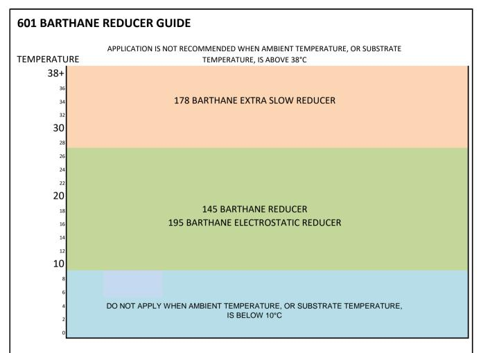
This chart is provided as an approximate guide to when the different thinners should be used. Differences in application technique and the size of the components being painted will influence the optimum thinner choice.
