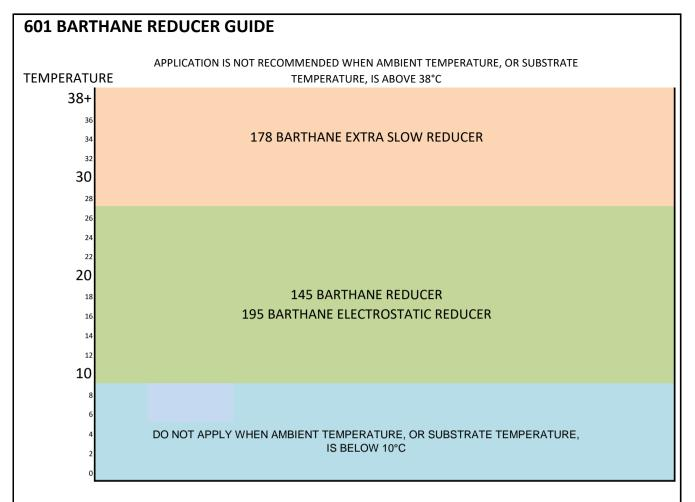
This chart is provided as an approximate guide to when the different thinners should be used. Differences in application technique and the size of the components being painted will influence the optimum thinner choice.
